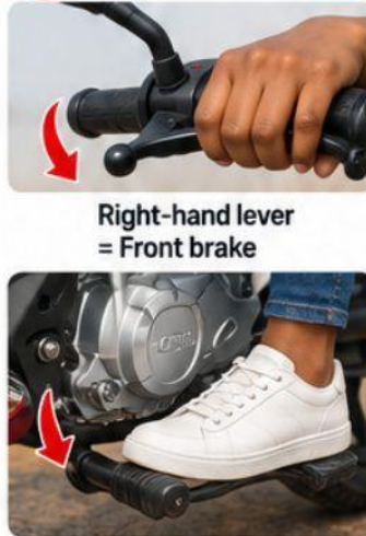
Right-foot pedal = Rear brake
